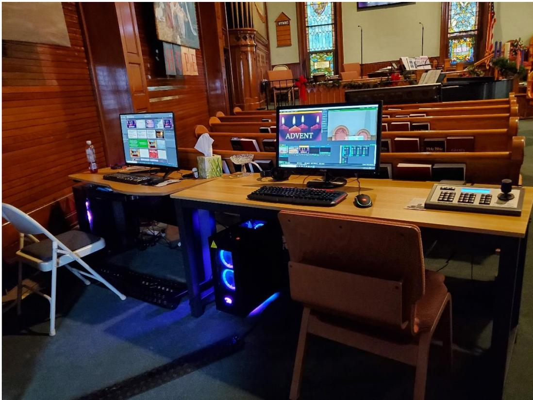
The joystick in the image above is used to control two PTZ cameras (see pictures below) that capture images from two distinct vantage points. This has enabled us to broadcast higher quality and more focused video of the pulpit, communion table,
